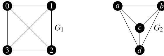
Figure 1.3: The graph G_1 is isomorphic to G_2 , since there exists a bijective mapping \phi: V(G_1) \mapsto V(G_2) s.t. \phi(0) = a, \phi(1) = b, \phi(2) = c, \phi(3) = d and \forall (u, v) \in E(G_1) \Leftrightarrow (\phi(u), \phi(v)) \in E(G_2) .
